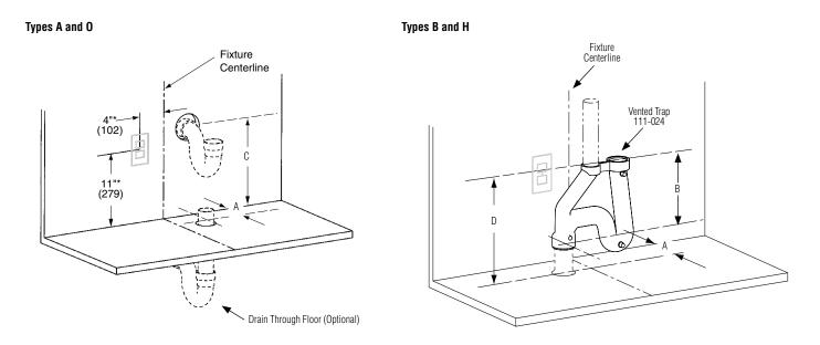
\* Suggested location of 120VAC GFCI electrical outlet. Always check local codes before installing. Outlet may be required to be in a remote location.
