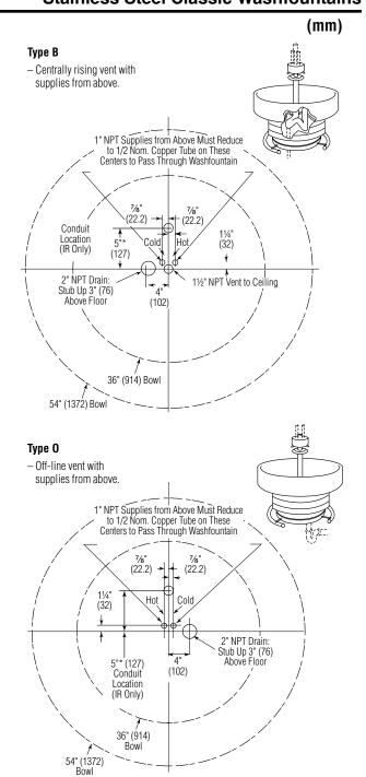
\* Remote mounting of plug-in adapter with 120 VAC electrical supply to washfountain is recommended. See local electrical codes before roughing in. (This conduit location is only a recommendation.)
