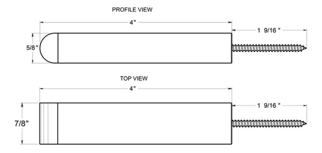
Notice: Top and Profile Views are relative to the installation, this product can be installed either way.
