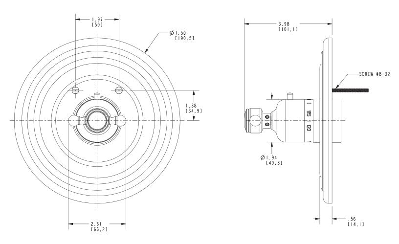
NOTE: Product Dimensions for the Shower System Control Valve Handle Trim (Handle/Escutcheon can be found within the Spec Sheet for that specific part number.
