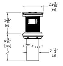
THROUGH-HOLE SPECIFICATIONS RECOMENDED MIN <u>MAX</u> SPOUT: Ø1" [25] VALVE: Ø1" [25] Ø 1-1/2" [38] Ø 1-1/2" [38] Ø 1-3/8" [35] Ø 1-3/8" [35]
