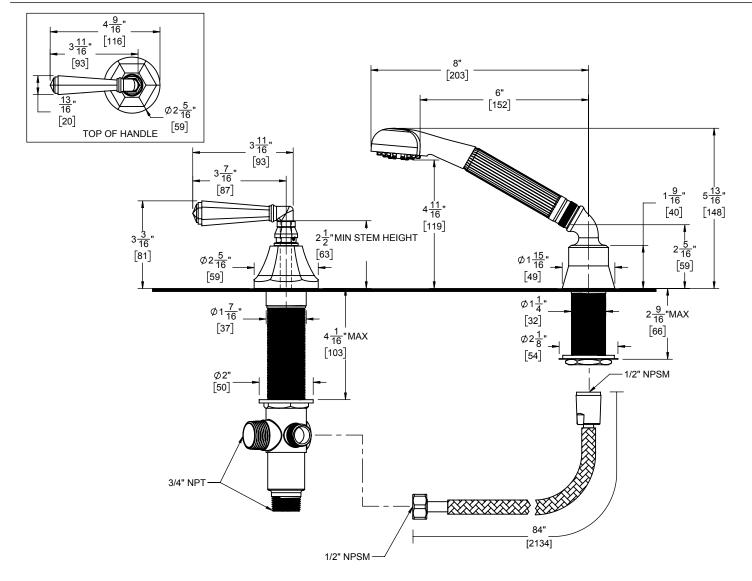
THROUGH-HOLE SPECIFICATIONS **RECOMENDED** MIN <u>MAX</u> SHOWER: Ø1-1/4" [32] VALVE: Ø1-7/16" [37] Ø 1-1/4" [32] Ø 1-1/2" [38] Ø1-11/16" [43] Ø1-3/4" [44]
