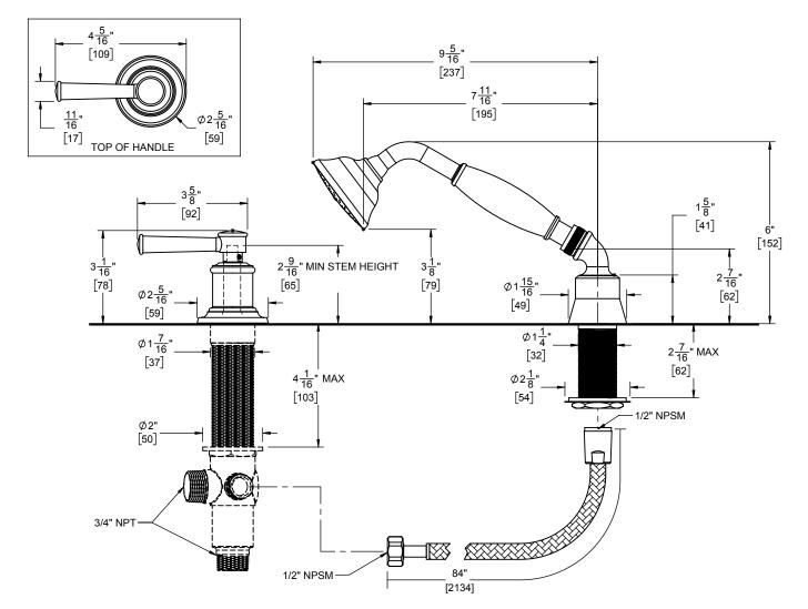
**THROUGH-HOLE SPECIFICATIONS** RECOMMENDED <u>MIN</u> **MAX** SHOWER: Ø1-1/4" [32] VALVE: Ø1-7/16" [37] Ø1-1/4" [32] Ø1-1/2" [38]
