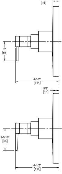
Dimensions are inches, rounded to 1/16" [Dimensions in brackets are mm, rounded to 1mm]
