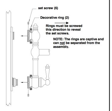
**Important note:** If the set screw points are not properly seated into the "V" groove, the tops of the set screws will not allow the decorative rings to be threaded into place – **this is a safety feature that assures a proper connection to the pipe adapter.**
