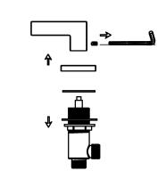
2. Remove mounting hardware from handle body. Connect water supply tube to valve body and tighten with lock nut. Do not allow the water supply brass tube to twist. Use two wrenches, as shown in the diagram, tighten the flexible hose.
