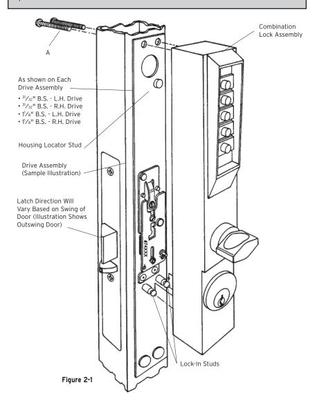
B-2 Fix two each 10-24 x 2 1/8" long round head machine screws (A) as shown (See Figures 2-1 & 2-2). Using the DF-59 key, thread the control lock assembly (B) into the combination change sleeve (C) DF-59 (See Figure 2-2) until trim plate is snug against stile. The key can only be removed in vertical position.
