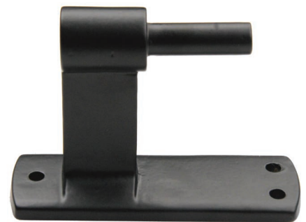
Pintle on Plate - 2-1/4" Offset S4-420-19 Dimensions: 3-1/2" L x 1-1/4" W Offset: 2-1/4" Screw: 1" Round | #10
