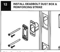
Using the reinforcing strike as a guide, predrill the screw holes. Install dust box and reinforcing strike. Ensure 3" screws for reinforcing strike are installed on the stop side of the plate.
