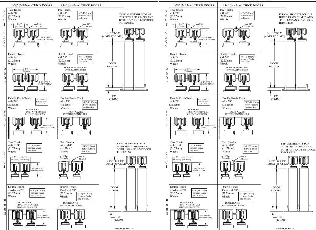
FLOOR CLEARANCE: Allow 1/2" (12.7mm) between door and finished floor.
