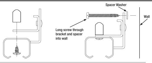
Door Weights from 100 to 150 lbs. (9821 Track): If the door weight is greater than 100 lbs., and not more than 150 lbs., secure side wall mount brackets to wood header and studs on 16" centers as well as at both ends of the track.
