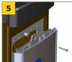
To mount to a bollard, attach the switch to the bollard using a 10-24 x 0.75 mounting screw and nylon spacer.
