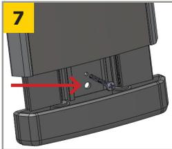
Secure the plate assembly using the bottom mounting screw.
