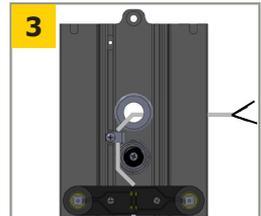
Make necessary wiring connections.<sup>2</sup> Ensure excess wiring is kept inside the junction box, if used.<sup>3</sup>
