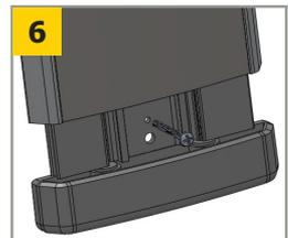
To secure the bottom plate assembly, first slide the front plate upwards, and then insert a top end cap screw into the threshold to hold.
