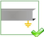
The door control system and the header cover profile must be correctly grounded.
