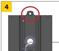
Install an appropriate anchor through the top mounting hole.
