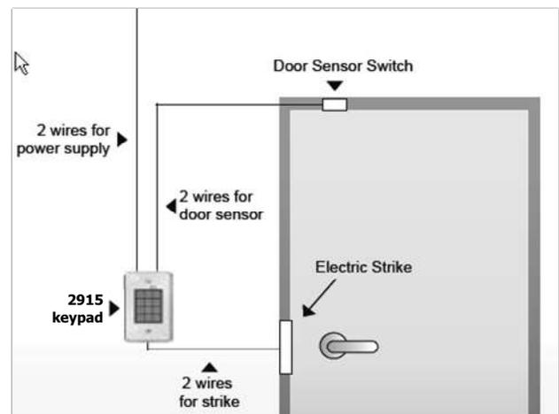
Fig. 3 Basic Door Installation
