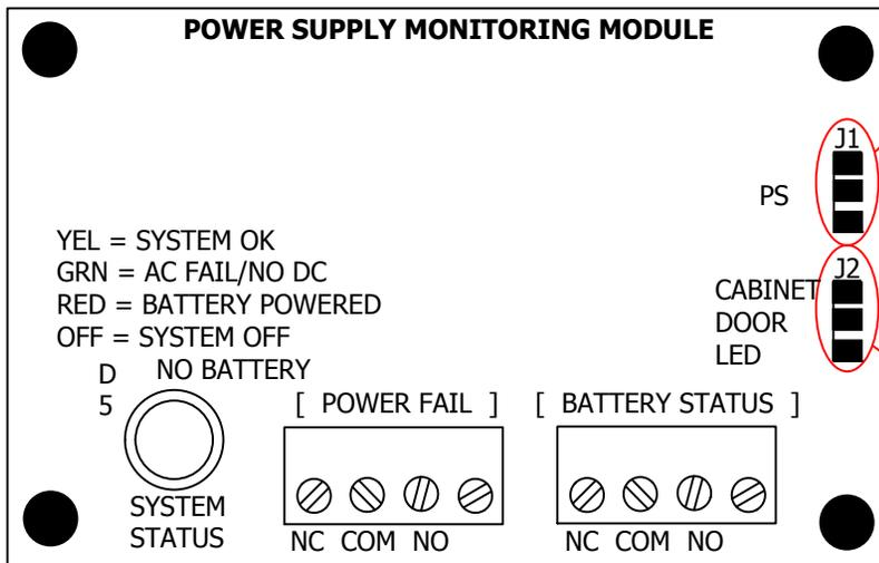
Attached one end of cable supplied with the monitor module to J1. Attach the other end to J6 on the power supply circuit board.
