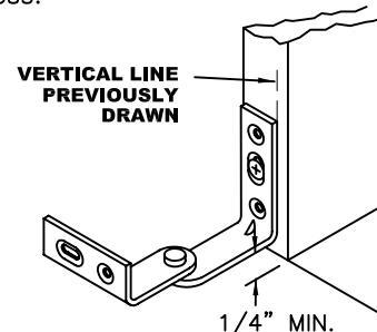
Apply bottom hinge to face of mullion using the center of the elongated hole. Be sure to line up with previously drawn vertical line.
