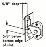
Hold strike so stamped lines on strike are level with top edge of hook. Mark slot outline with pencil. Cut mortise into jamb as shown.
