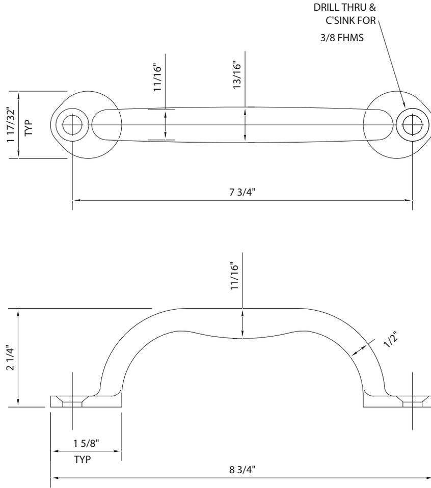
DO NOT SCALE THIS DRAWING -- TOLERANCES ON FRACTIONS ±.015" ON DECIMALS ±.005" EXCEPT AS NOTED
