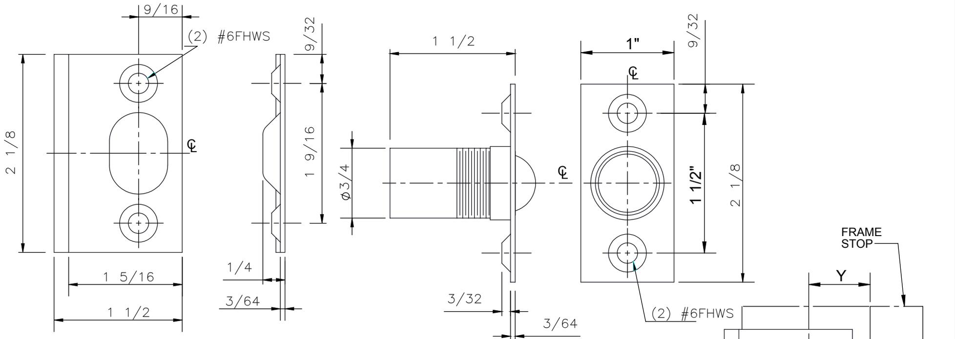
1. CHOOSE HEIGHT AT WHICH TO MOUNT HARDWARE AND MARK AN "X" ON THE DOOR EDGE. (MAKE SURE "X" IS IN THE CENTER OF THE DOOR EDGE BEFORE GOING ON.)
