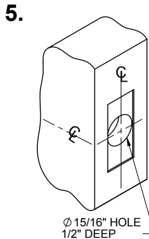
5. DRILL 15/16" DIAMETER HOLE 1/2" DEEP IN CENTER OF THE MORTISE
