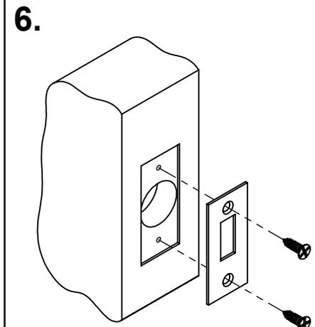
6. SCREW STRIKE PLATE INTO POSITION USING (2) #6 x 3/4" FPHWS.
