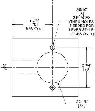
**NOTE:** INSERT LATCH INTO  $\phi$ 1" [25] HOLE USING FINGER PRESSURE. THEN WHILE HOLDING A PIECE OF WOOD OVER THE LATCH FACE, STRIKE WITH A MALLET UNTIL LATCH IS SITTING FLUSH WITH DOOR EDGE.
