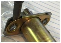
While holding the latch, twist the screwdriver to pry the face plate off the mounting bracket.
