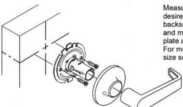
Measure centerline of lock height as desired from finished floor. Measure backset as desired from door edge and mark centerline. Press mounting plate against door and tighten screws. For metal doors, drill and tap for #8-32 size screw. Press on rose and handle.
