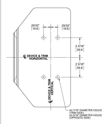
**STEP 1.**PREPARE PUSH SIDE OF THE DOOR FOR EXIT DEVICE. SEE EXIT DEVICE TEMPLATE FOR DOOR PREPERATION DETAIL.
