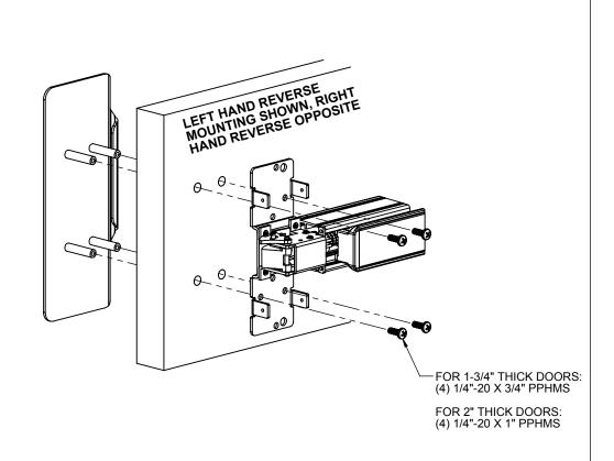
**STEP 3.**SECURE PULL AND EXIT DEVICE USING THE 4 MOUNTING SCREWS.
