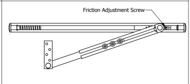
Using a flat head screw driver, turn the friction adjustment screws clockwise to increase the friction and counter-clockwise to lower the friction.
