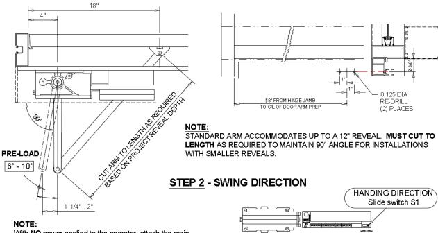
With  $\underline{\text{NO}}$  power applied to the operator, attach the main arm to the motor allowing for a minimum of  $6^\circ$  pre-load and pull against motor resistance to make the final  $90^\circ$  connection to the door portion. Arm spindle adaptor has splines to allow for adjustment in  $6^\circ$  increments.
