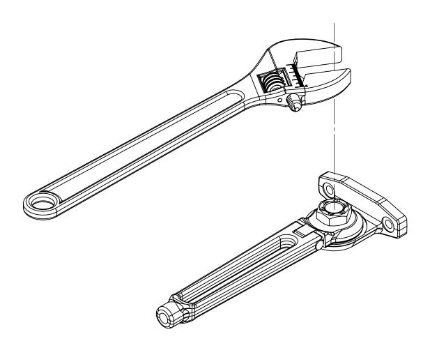
Meant to be used in scenarios where the door is held open infrequently, friction hold open arms may require occassional maintenance after multiple engagements. Should the hold open function become loose, open the door to the desired angle of hold open and tighten as shown.
