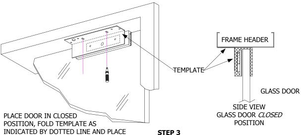
POSITION, FOLD TEMPLATE AS INDICATED BY DOTTED LINE AND PLACE TEMPLATE AGAINST FRAME HEADER AND BRACKET THEN MARK AND DRILL AS INDICATED.
