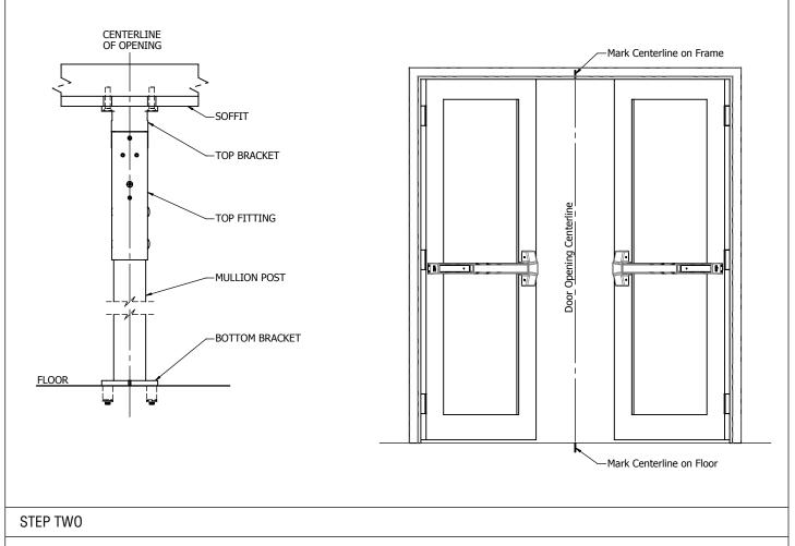
Measure and mark a centerline on the width of the top bracket.
