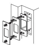
Match screw holes on strike with vertical centerlines on jamb. Mark outline of strike and chisel 1/4" (6.4mm) deep for flush fit of dust box, wood frame reinforcer, and strike. Place dust box and wood frame reinforcer into mortised area and tighten to the frame using 3" wood screws. Insert the strike and tighten to the frame with #8 screws.
