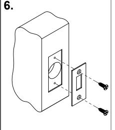
SCREW STRIKE PLATE INTO POSITION USING (2) #6 x 3/4" FPHWS.
