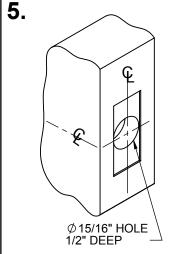
DRILL 15/16" DIAMETER HOLE 1/2" DEEP IN CENTER OF THE **MORTISE**
