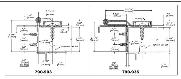
HAGER Models 790-903 and 790-935 are Stainless Steel Continuous Half Surface Hinges for 1-3/4" (44.5mm) thick doors. Clearance required between the hinge edge of the door and the frame rabbet is 1/8" (3.2mm) minimum. Both models provide for a 1/8" door inset. Model 790-935 provides 'swing clear' rotation.
