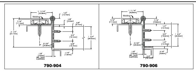
HAGER Models 790-904 and 790-906 are Stainless Steel Continuous Half Edge Mount Hinges for 1-3/4" (44.5mm) thick doors. The frame face must have a flat surface at least 1-5/8" wide. Clearance required between the hinge edge of the door and the frame rabbet is 1/8" (3.2mm) minimum. *Model 790-906 features an integral protective corner guard and is not recommended for use on doors that have a beveled edge on the hinge side*.
