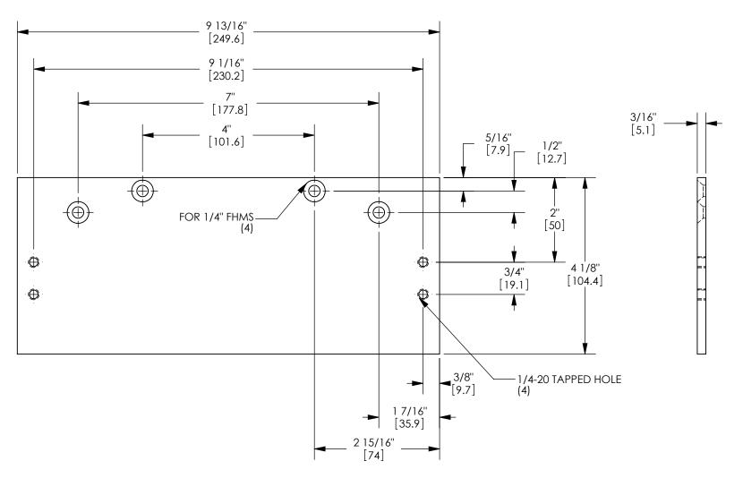
SCREW PACK INCLUDES: 4 PCS: 1/4-14 x 1-1/2" FPHS SELF DRILLING (STEEL) 4 PCS: 1/4-20 x 1-1/2" FPHS SELF DRILLING (STEEL) 4 PCS: 1/4-20 x 7/16" OPHS (STEEL)
