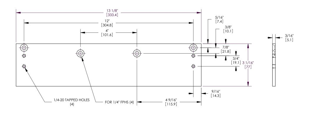
SCREW PACK INCLUDES: 4 PCS: 1/4-14 x 1-1/2" FPHS SELF DRILLING (STEEL) 4 PCS: 1/4-20 x 1-1/2" FPHS SELF DRILLING (STEEL) 4 PCS: 1/4-20 x 7/16" OPHS (STEEL)
