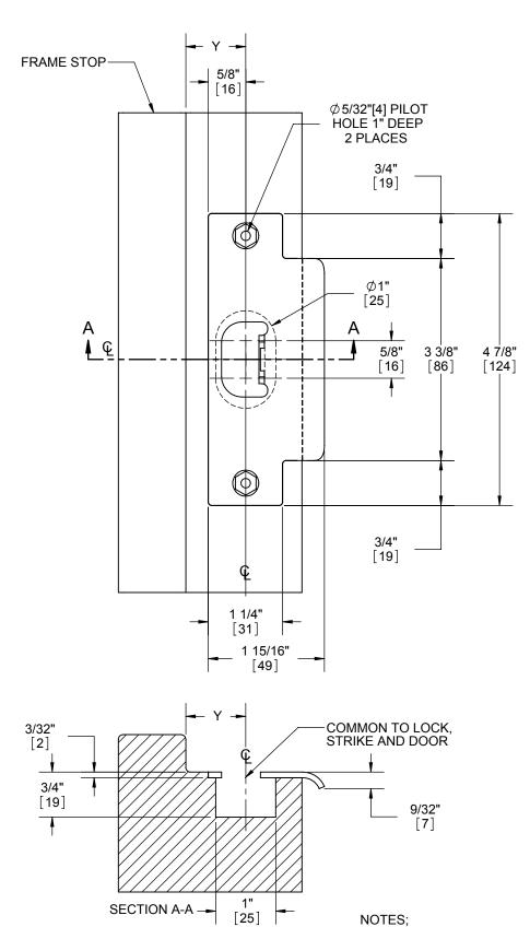
DIMENSION "Y" IS A FUNCTION OF DOOR THICKNESS. 1. STRIKE LOCATION MUST BE CHANGED RELATIVE TO THICKNESS OF DOOR SILENCER OR 2.
