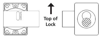
Fig. 3b - Back of door lock with bolt installed
