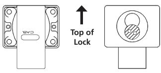
Fig. 3a - Back of drawer lock with bolt installed.
