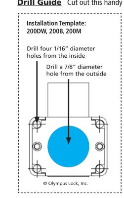
**Drill Guide** Cut out this handy drill guide for easy installation.
