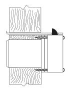
**Note:** Strike must be lined up so that dead lock portion of latch is depressed when drawer is closed.
