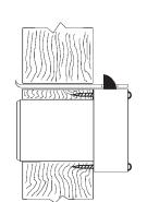
**Strike installation:** Line up center mark on latch with center mark on strike for correct strike placement.
