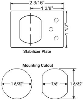
Lock diameter is 1-1/8". Drilled hole should be slightly larger.
