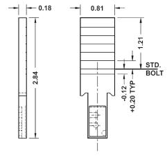
**T37-2** Long bolt can be cut to length required by application
