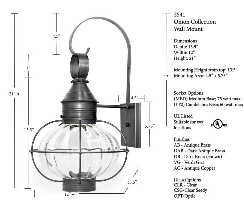
Also includes Brass mounting nipple and steel mounting bracket. Brass mounting bracket available upon request. Thumbscrews are brass and bottom globe/cage can be removed for easy cleaning or bulb replacement.
