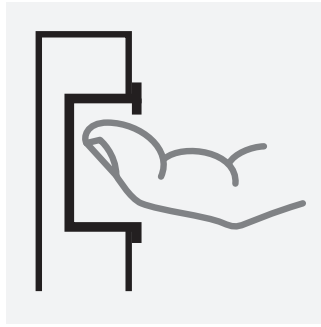
Flush/Recessed Pull - Lip at Top Install with screws from back or glue in; panel routed out from front.
