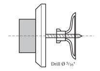
FASTENERS NOTE: Sheet Metal Screw & Toggler
