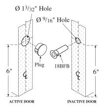
IMPORTANT: The 18BFB will project during a fire. Do not cover with any edge mounted door hardware.
