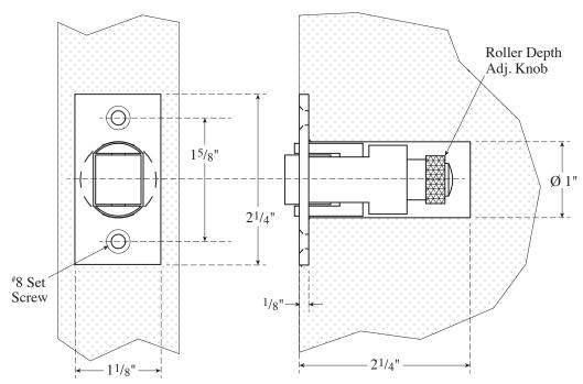
The roller latch can be mounted into the door and the strike into the frame or the strike can be mounted into the door and the roller latch into the frame depending on individual choice. Side jamb or header mounted.
