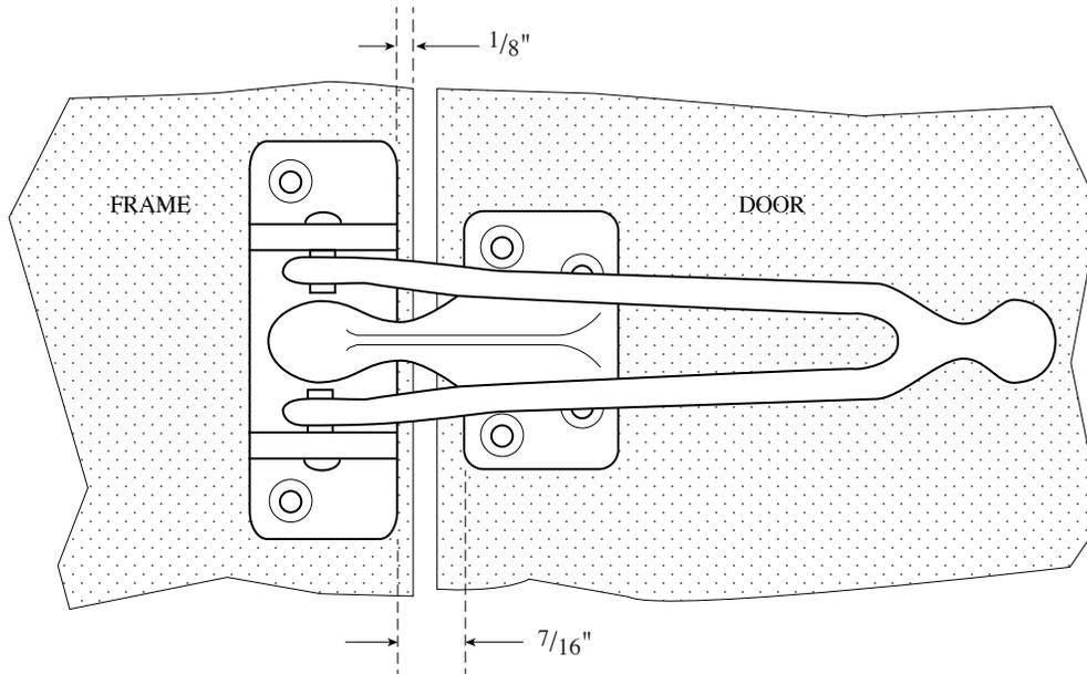
Note: The door guard should be mounted approximately 54" above the floor. (Check with your local authority for any special ADA requirements).
